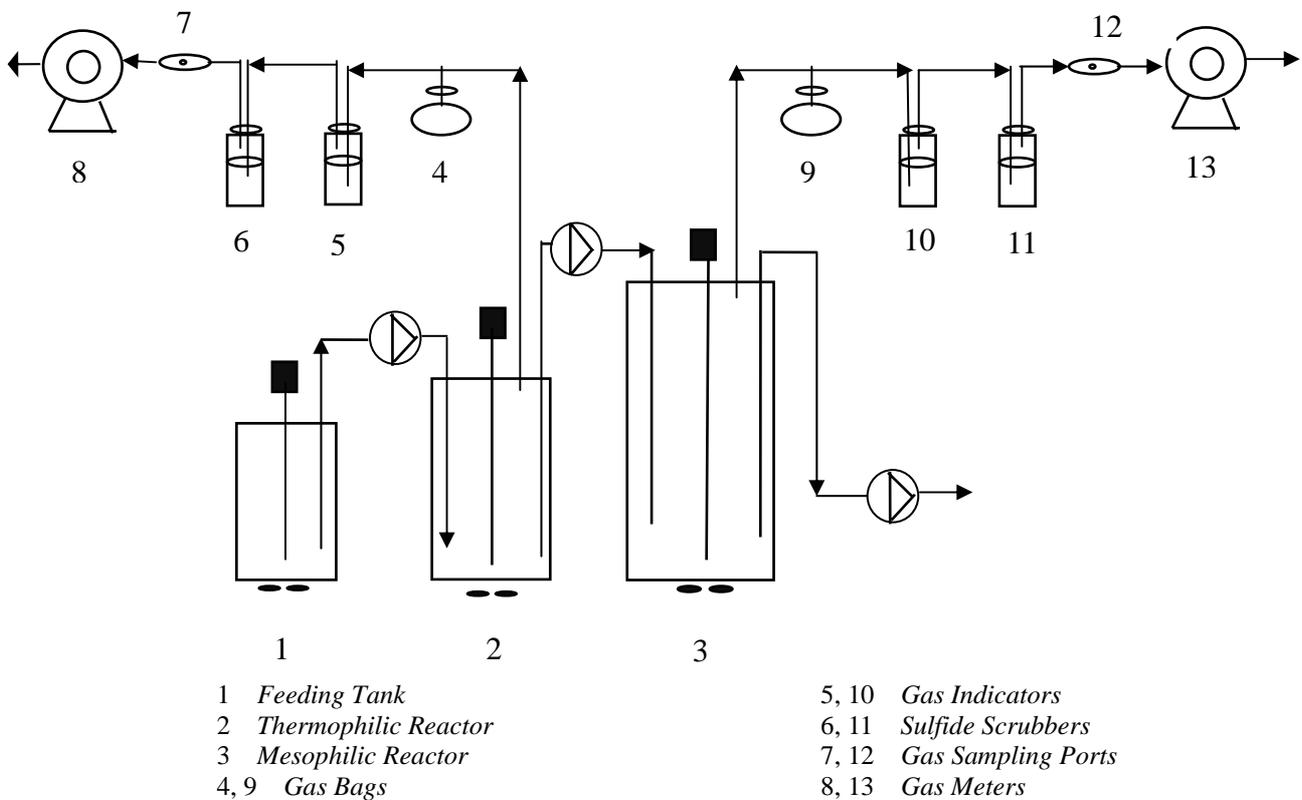
Figure 1. Schematic of the TPAD system
