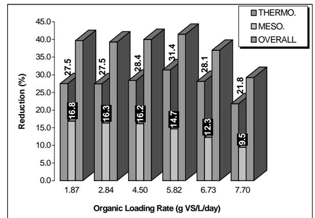
Figure 2. Individual reactor and system volatile solids removal at different organic loadings
