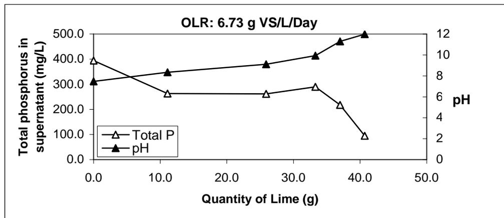
Figure 4. Phosphorus removal by lime
