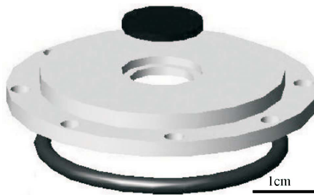
Figure 3. Drawing of the chamber of the measurement device.
